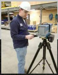
Our scanning crew in the field at the end of November in Big Lake! We were scanning fabricated material to make sure they are the correct dimensions before shipping off to the slope! >>CHRIS BURT
